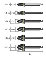
\* Note: Drill speed 1,000rpm, 30~45 N·cm with irrigation
