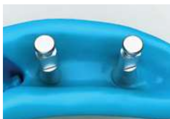
Connect analogs with the embedded impression coping.
