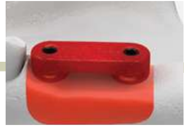
Fabricate the positioning jig
